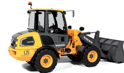
Electric wheel loader
